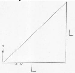
**a.** (7 points) TM fields. In terms of the mode indices (n,m) for the related square waveguide of side L, find the longitudinal TM fields.
