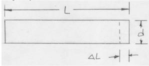
**d.** (10 points) Shape perturbation. The resonator is restored to length L. Now suppose the upper plate of the resonator is perturbed in shape by adding a conducting rectangular bar of length  $\Delta L$  and height  $\Delta d$  across the full width w at the center of the resonator as shown. Find the corresponding change in the angular frequency of oscillation. (You can assume  $\Delta d \ll \Delta L \ll d$ , L.)
