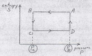
The reversible Brayton engine cycle  $A \rightarrow B \rightarrow C \rightarrow D \rightarrow A$  is shown in the entropy-pressure (S-P) diagram. During step  $D \rightarrow A$ , the gas is heated at constant pressure with the absorption of an amount of heat  $Q_{DA}$ . During step  $B \rightarrow C$ , the gas is cooled at constant pressure with the expulsion of an amount of heat  $Q_{BC}$ .
