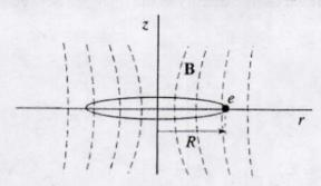
In a betatron, electrons are accelerated by a magnetic field which changes with time. Let  $\langle B \rangle$  equal the average value of the magnetic field over the plane of the orbit (within the orbit), i.e.  $\langle B \rangle = \frac{\Phi}{\pi R^2}$ , where  $\Phi$  is the magnetic flux through the orbit. Let  $B_0$  equal B(r=R,z=0)
