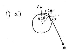
Since the string extends tangentially to the disk, the geometry is as shown in the figure.
